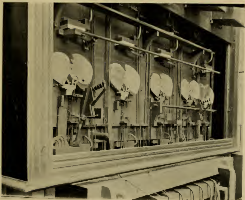
Part of the "action" of a keyboard colour-organ, with colour-producing diaphragms removed.
