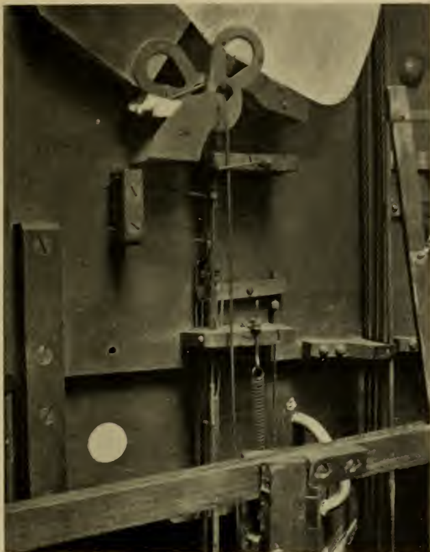
Part of the "action" of the inner diaphragms for giving intervals of relative strength in the colour for each octave.
