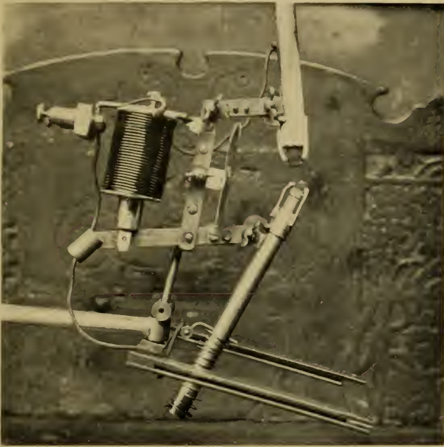
One of the patterns of arc-lamp, specially designed for mobile colour instruments.
